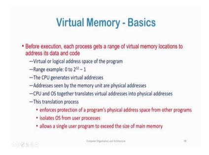
Now virtual memory allows the main memory to be shared between multiple programs. Before execution each process gets a range of virtual memory locations to address its data and code. So, as we are talking this is virtual memory it does not exist in practice.
