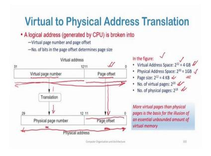
So, virtual to physical address translation a logical address generated by the CPU is broken into a virtual page number and a page offset. So, here I said that my if in let us say I have a 32 bit address space, 32 bit address bus. So and I have a 32 bit virtual address space, so, my virtual addresses will be of length 32 bits in this figure we see that the virtual address or also called the logical address is broken into 2 parts the virtual page number and the page offset.
