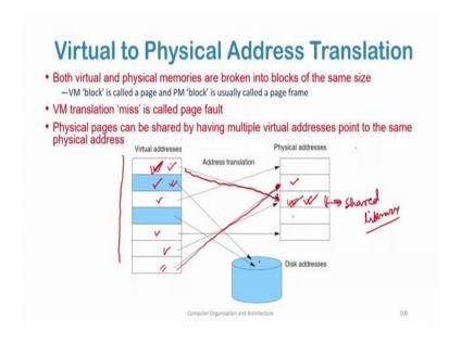
Now how do we do this mapping from virtual to physical addresses? So, both the virtual and physical both the virtual and physical memory; so the virtual memory and the physical memory are broken into blocks of the same size and this block. So the blocks are of the same size. As for caches we divide into blocks and lines for virtual memories. And physical memories we divide virtual memory into blocks called pages and the physical memory into blocks of the same size called page frames.
